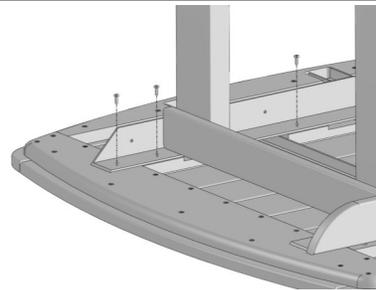
Flip over Base Assembly and align Aluminum with cleats on the Table Top Assembly. Secure using (20) 3/4" Pan Head Screws.
