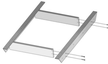
Align predrilled holes in Short Aprons with holes in Aluminum Support Brace as shown. Secure using (8) 1 3/4" Phillips Head Screws.
