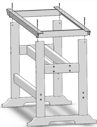
Align large holes in Aluminum Support Braces with Predrilled holes on outside corners of Legs as shown. Secure using (4) 80mm Hex Lags.
