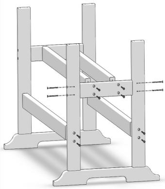
Attach Stretchers to Leg Assemblies using (24) 80mm Hex Lags (8 for Dining Height) as shown. Plug holes with 5/8" Bungs using Rubber Mallet.
