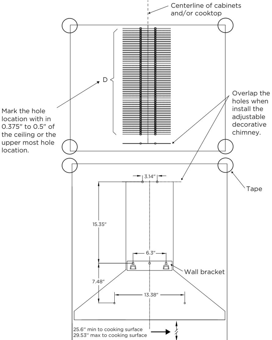
NOTE: Ensure that horizontal lines are level prior to marking hole locations.
