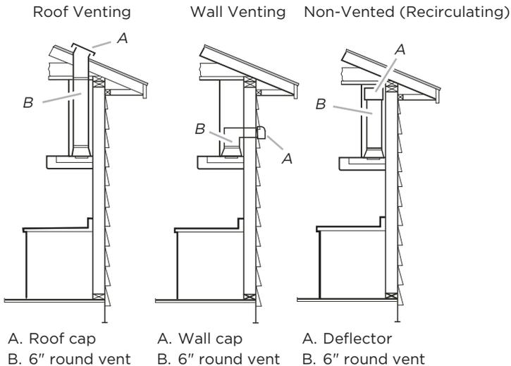
Local building codes may require the use of makeup air systems when using ventilation systems greater than specified CFM of air movement. The specified CFM varies from locale to locale. Consult your HVAC professional for specific requirements in your area.
