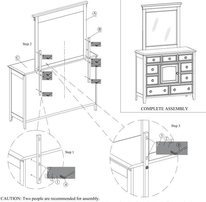
Step 1: Secure batten to the dresser using flat washer (3), spring washer (2), allen bolt (1) and allen wrench (4).
