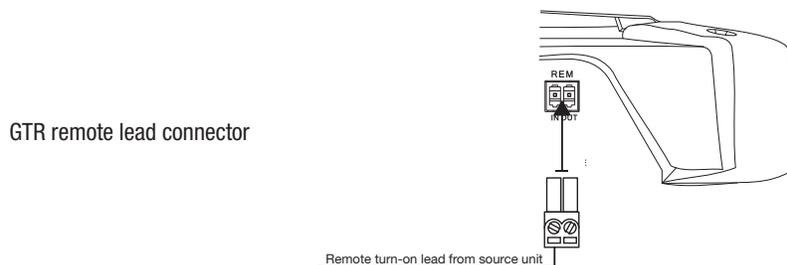
In addition to REM inputs that turn on the amp, there are REM outputs that can be used to turn on other amps. If the amp auto turns on when detecting a Bluetooth signal or ADAS input, its REM outputs will turn on the other amps as well.
