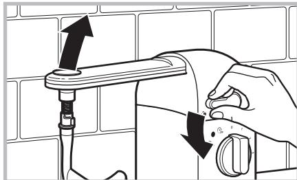
2. Raise the stir arm by pressing down on the release lever.
