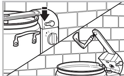
6. Once cooking is complete, set the Stir Tower to 0 (OFF). Press down on release lever and raise stir arm before removing cooking pot.
