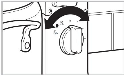
5. Add ingredients to Multi-Cooker and cover. Once cooking mode is set and started (see Multi-Cooker instructions), select desired stir speed or intermittent stir mode. Power on indicator will light.
