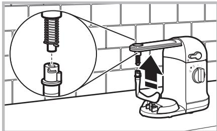
1. Align pins on Stir Tower shaft with slots on flip-and-stir wand. Press up and rotate counterclockwise to lock into place.
