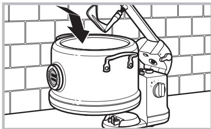
3. Align back of Multi-Cooker with front of Stir Tower. Lower Multi-Cooker onto easy connect power port on Stir Tower base.
