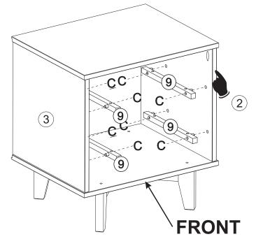
Use screw (C) to attach parts (9) to parts (2,3) *NOTE*: The extra holes in part (9) should face the top of parts (2,3)
