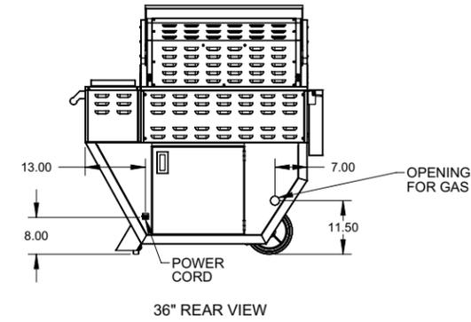
**GAS REQUIREMENTS:** 1/2" NPT gas connection. Minimum gas supply is 7" water column for natural gas and 11" for propane. Operating pressure at the manifold is 4" water column for natural gas and 10" for propane. All units require a regulated gas supply. (included)
