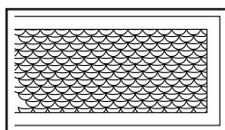
For best performance: Replace grease filters with half-moon openings facing out - and in orientation shown.
