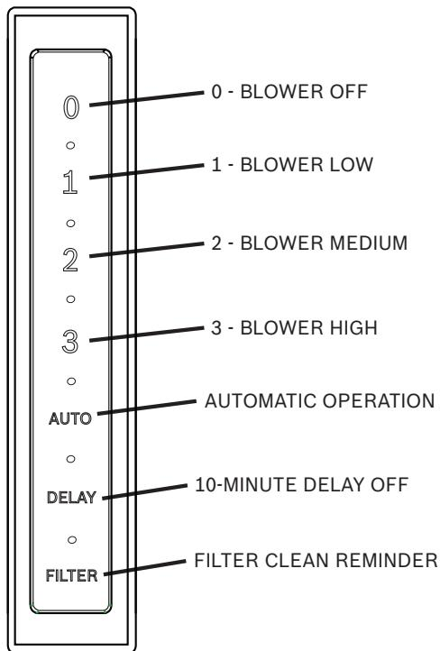
All hood controls, located on the right side panel of the intake housing frame, are visible when the hood is raised.
