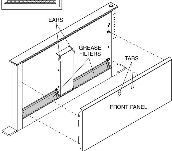
Remove front panel and take out the (2) grease filters.
