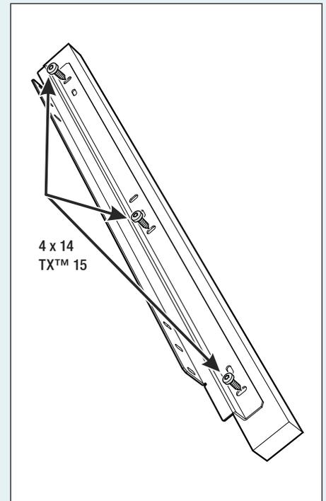
Mount the panel onto the angle bracket using three 4 x 14 screws.
