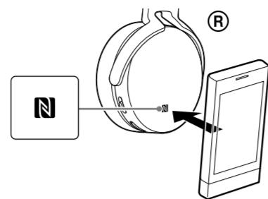
By touching the unit with a smartphone, the unit is turned on automatically and proceeds to pair and connect via BLUETOOTH.
