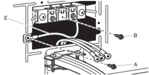
Install the correct strain relief for your electrical connection method. Remove center terminal block screw (B). Remove neutral bond wire (E) from green external ground conductor screw (A).
