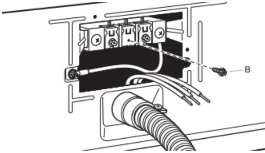
Remove center terminal block screw (B).
