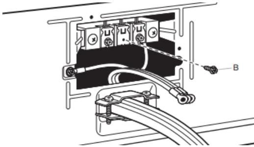
Remove center terminal block screw (B).
