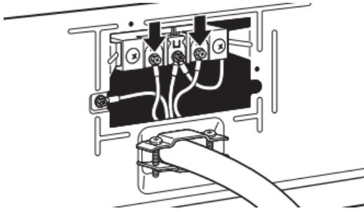
Connect remaining wires under outer terminal block screws. Tighten screws. Insert tab of terminal block cover into slot of dryer rear panel. Secure cover with hold-down screw. Now, go to "Venting Requirements."
