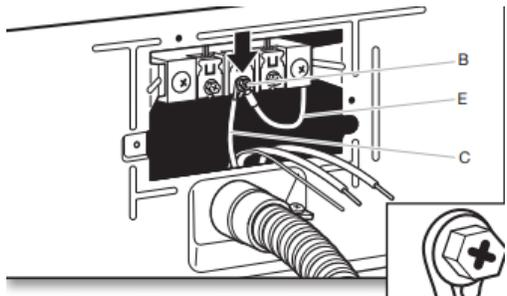
Connect neutral bond wire (E) and place hooked end (hook facing right) of neutral wire (white or center wire) (C) of direct wire cable under center screw of terminal block (B). Squeeze hooked ends together and tighten screw.
