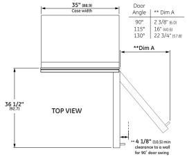
\*\* These refrigerators are equipped with a 3 position door stop. The factory set 1.15° door swing can be adjusted to 90° if clearances to adjacent cabinets or walls is restricted. Allow full 130° door swings for pan removal. If the 90° door stop position is used, pan access is maintained, but pan removal is restricted.
