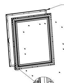
Step: 7 Remove the Front Panel from the Door Assembly by removing the inner mounting screws, 4 per side, from the perimeter of the assembly. Rotate the Front Panel 180°, the top becomes the bottom. Reattach using the same
