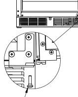
Step 13: Lift the-Door Assembly and insert top pin into bearing. Then move door toward cabinet and align V-Blocks.
