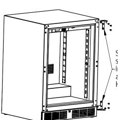
Step 5: Using the screws from Step 3, install the new Top and Bottom Cabinet Hinge Brackets.
