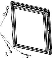
Step 12: Place Lower V-Block into Lower Cabinet Hinge with notch parrallel to cabinėt.
