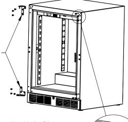
Step 4: Remove the Hole Plugs from the Top and Bottom Hinge Bracket mounting holes. Then place them in the holes on the opposite side made vacant in Step 3.
