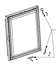
Step 6: Remove the Top and Bottom Door Hinge Brackets and the Push Plunger Bracket. Save the screws for later.
