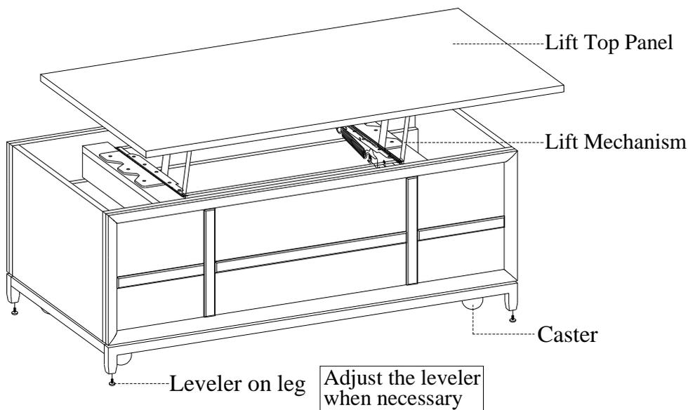
Adjust the leveler when necessary
