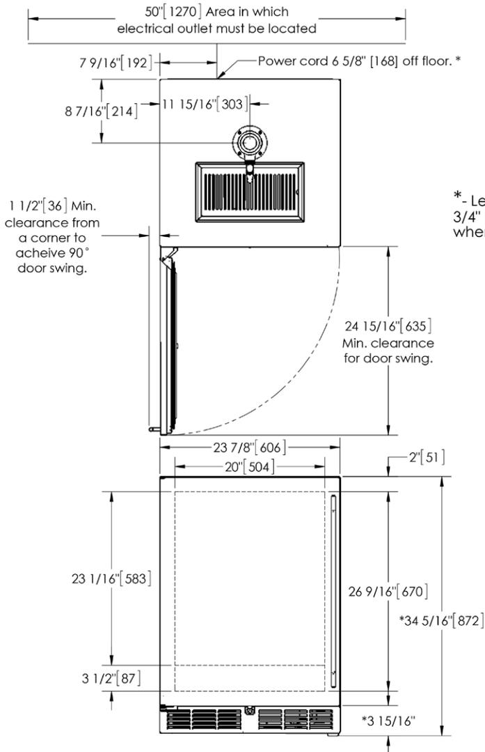
\* - Leg leveler can add 3/4" [19] to these dimensions when fully extended.
