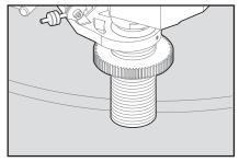
Place masking tape over cartridge guard to hold it in place. Remove tonearm and wrap in supplied plastic bag. Place tonearm securely in foam top cutout.
