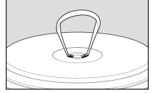
Install platter strap and thumb screws. Lift platter from turntable and wrap in supplied plastic bag. Place the platter securely in the foam base.
