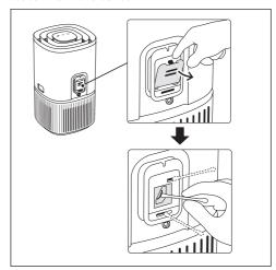
After having cleaned the sensor box, we recommend to vacuum clean the filter at the same time.
