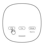
NOTE: When turning ON the air purifier, it will take about 10 seconds for the sensors to calibrate and analyze the air quality. During this time, the air quality indicator will pulsate slowly in white.
