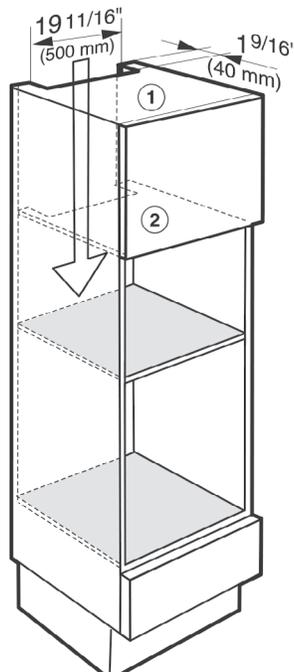
To ensure that the Combi Steam Oven has adequate ventilation, the following cut-outs measuring 19 1/16" x 1 9/16" (500 x 40 mm) must be made:
