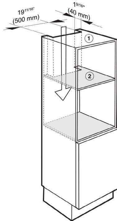
To ensure that the Combi Steam Oven has adequate ventilation, the following cut-outs measuring 19 11/16" x 1 9/16" (500 x 40 mm) must be made:
