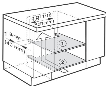
To ensure that the Combi Steam Oven has adequate ventilation, the following cut-outs measuring 19 11/16" x 1 9/16" (500 x 40 mm) must be made:
