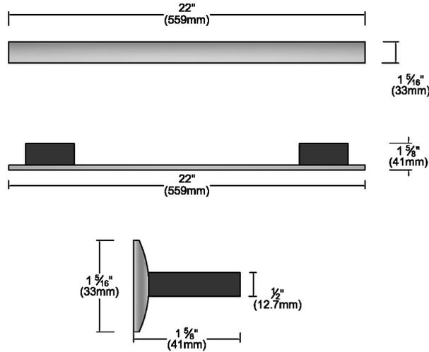
Please note hinges may require adjusting or replacing when changing from a ContourLine Handle to a PureLine or Miele Signature Handle.
