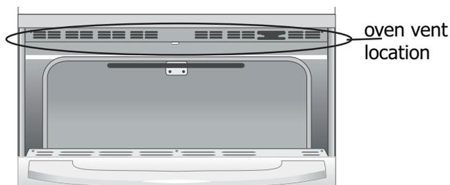
Figure 1: Do not block oven vent location
