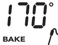
**Figure 20: Probe set showing meat probe temperature**
