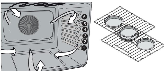
**Figure 14:** Rack positions and suggested pan placement [Figure 14](#)
