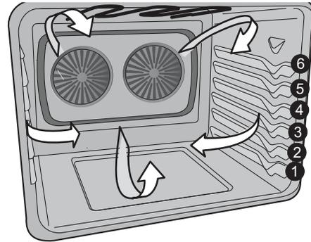
Figure 16: Convection roasting on lower oven racks
