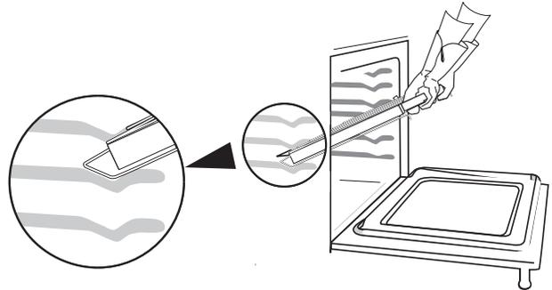
**Figure 5: Remove and replace using both hands**
