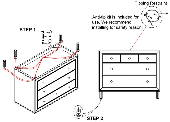
Adjust leveler if needed to level credenza on uneven floor.
