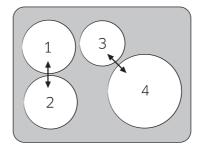
The cooking zones, which consist of paired cooking elements, are restricted to drawing a certain maximum amount of power. If you cause a cooking zone to exceed its maximum allowed power by switching on the Power Boost function, the Power Management function automatically reduces the power setting of the two elements in the cooking zone and reduces the power draw.
