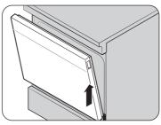
5. Lift door up and out until the hinge arm is clear of the slot (Fig. 2).
