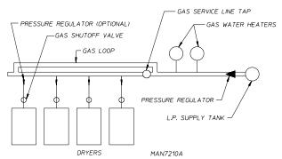
Consistent gas pressure is essential at all gas connections. It is recommended that a 3/4-inch (19.05 mm) pipe gas loop be installed in the supply line servicing a bank of dryers. An in-line pressure regulator must be installed in the gas supply line (header) if the (natural) gas pressure exceeds 13.0 in wc (32.34 mb) pressure.
