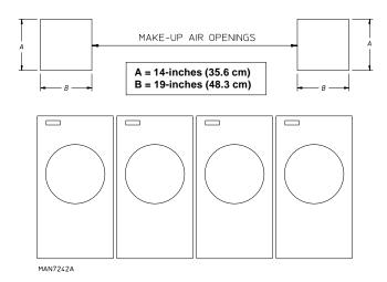
EXAMPLE: For a bank of four MDG78 dryers, two unrestricted openings measuring 14-inches by 19-inches (35.6 cm by 48.3 cm) are acceptable.
