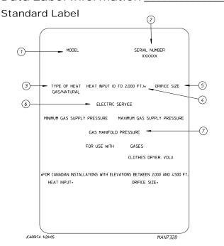
When contacting Maytag, the information on the data label is required to ensure proper service/parts assistance. The data label is located at the lower left rear of the dryer behind the back guard.
