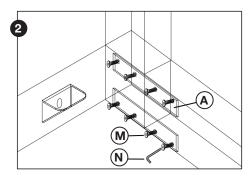
Use type A straight irons to connect the side rails and footboard
