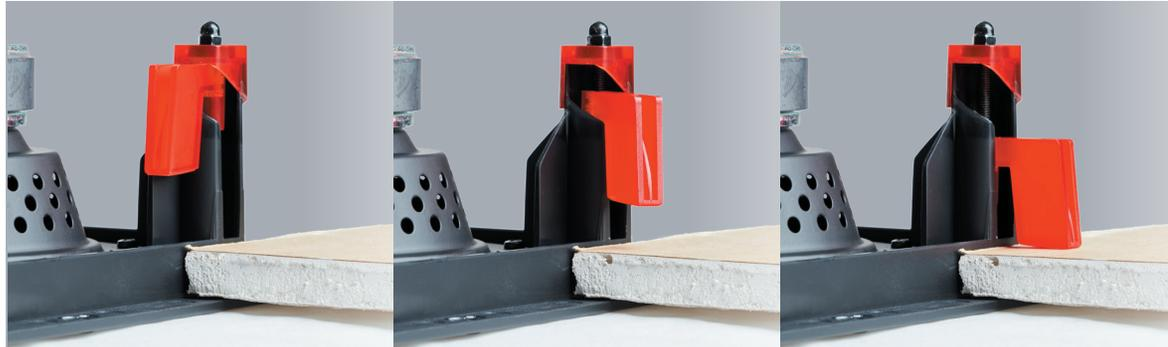
**USER-FRIENDLY INSTALLATION.** A simple, yet robust mounting-lock system allows quick, trouble-free installation. Pocketed screw holes help hold the drill steady, making installation a snap. When not in use, mounting locks are held securely within a self-contained housing. When moved into place, they couple the chassis firmly to the ceiling or wall, increasing the rigidity of surfaces. If ever removed, the locks retract and latch back in their housings.
