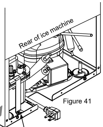
Remove the hex nut on rear drain pump bracket with the  $\frac{3}{8}$ " socket then remove the bracket.
