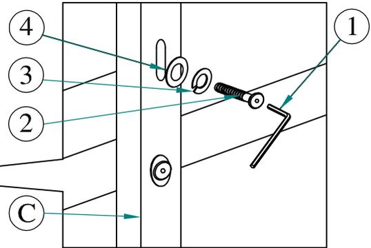
Step 1 / : Place mirror on the top of dresser as arrow shown. Align mirror to the center of dresser and tighten with (2) JCBC 35mm, (3) M6 Spring Washer & (4) Flat Washer. /
