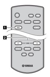
Press the **RADIO** source button to switch the audio source to FM.
