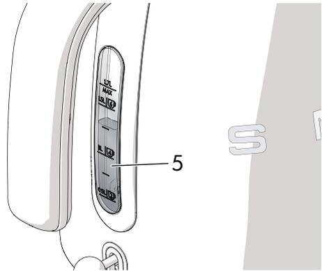
This indicator shows the level of water in the kettle, from the minimum fill level of 0.5 litres to the maximum of 1.7 litres, also showing the corresponding quantity in cups.
