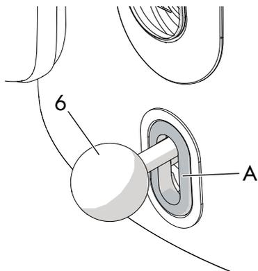
The ON/OFF lever starts or stops the boiling process. When the kettle is on, the LED **A** turns on and becomes white.
