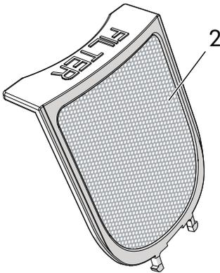
The stainless-steel filter is located behind the spout. It retains any scale present in the water.
