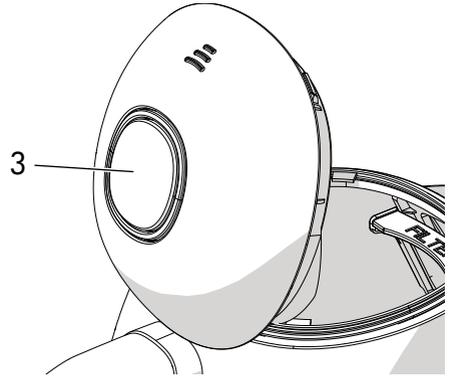
The lid has a push-push button (3) which allows it to open progressively to prevent the sudden release of steam.
