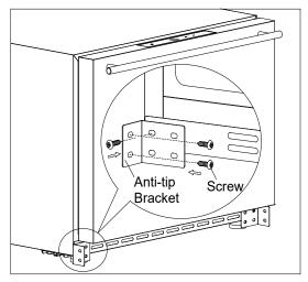
**NOTE:** If the unit is installed freestanding, please place the brackets in front of the unit's ventilation grille and secure the brackets to the surface it is being used on by the included screws.
