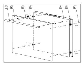
with a panel to fit the exact size of the drawer, remove the brackets (6) and the screws holding them to the drawer (7). Save the brackets and screws.
