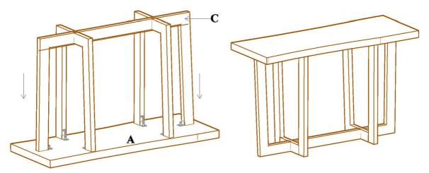
TIGHTEN ALL BOLTS FIRMLY AT THIS TIME USING ALLEN KEY (E). SET CONSOLE UPRIGHT.
