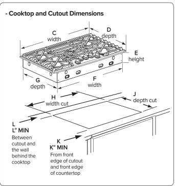
To ensure accuracy, it is best to make a template when cutting the opening in the counter
