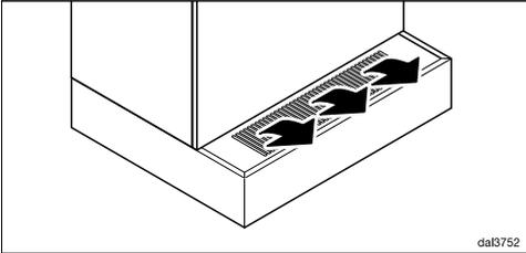
When selecting the installation position, ensure that the recirculation grille at the front of the appliance are not covered by the wall unit.
