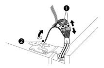
2 Rotate the hinge lever 3 counterclockwise. Lift the top hinge 4 free of the hinge lever latch 5.
