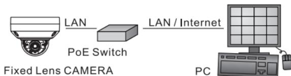
**(3). Use PoE power injector and the network switch connected to the network.**
