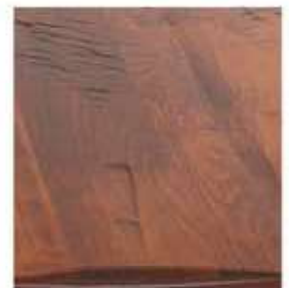
Maple, Elm, & Cherry have deeper cuts & Tear out
