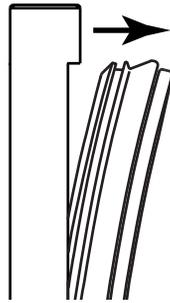
4. Upon removal, lay gasket down on a flat surface.
