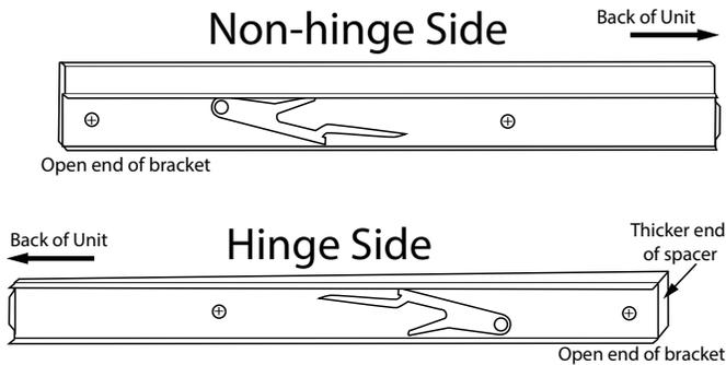
3. Line up rack slide with slide brackets and push rack in all the way. Pull rack outward all the way to make sure locks are engaged.
