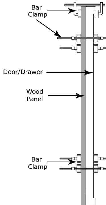
7. Using a 7/64" (3 mm) drill bit, drill 6 pilot holes into the wood panel 1/2" (12 mm) deep using the holes in the door frame as a guide.
