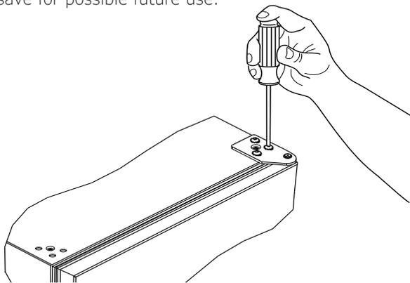
3. Remove door by tilting forward and lifting door off bottom hinge. Retain shoulder washers; they will be reused.
