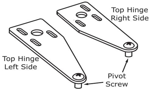
1. Remove pivot screw from hinge, flip hinge over, and install the pivot screw in the same hole from the opposite surface.
