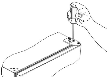
1. Remove door by tilting forward and lifting door off bottom hinge. Retain shoulder washers; they will be reused.
