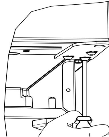
2. Remove corresponding screws on opposite side of cabinet. On some models there may be a nut behind one or both screws on either side.
