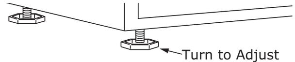
3. Confirm the unit is level after each adjustment and repeat the previous steps as needed.
