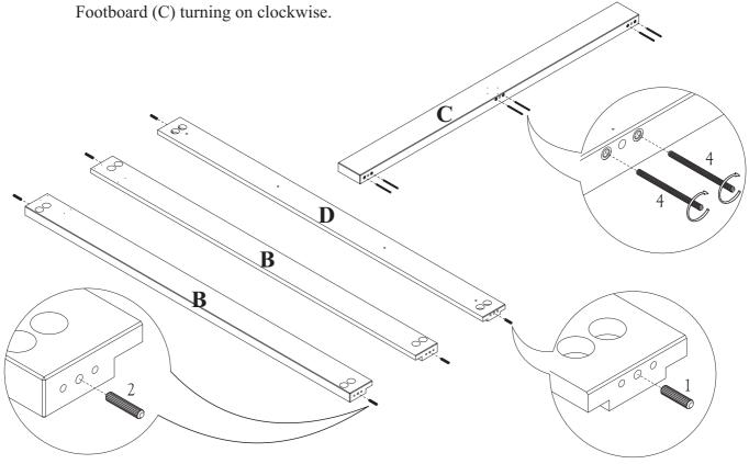
STEP 2: Attach the Side Rails (B) to Footboard (C) and fix with Elipse Nut (5) and Nut (6) tighten by Wrench (8).
