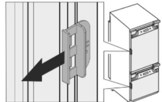
If the transport lock on the door is screwed on:
