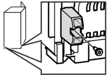
► Undo the screw and remove the spacers.
