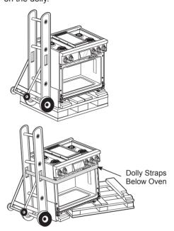
Transport the range on the furniture dolly close to its final location, tip the range back to level, and carefully remove the dolly.
