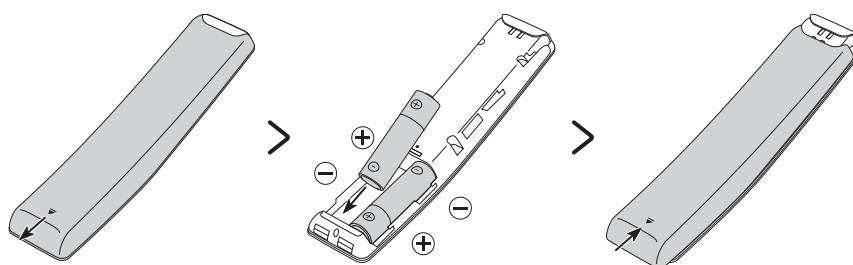
To install the batteries, push the rear cover open in the direction of the arrow at the bottom of the illustration, and then insert the batteries (1.5V AA type) as shown in the figure. Make sure that the positive and negative ends are facing in the correct direction. Close the rear cover as shown.
