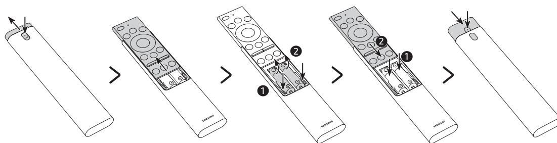
1. Press the
