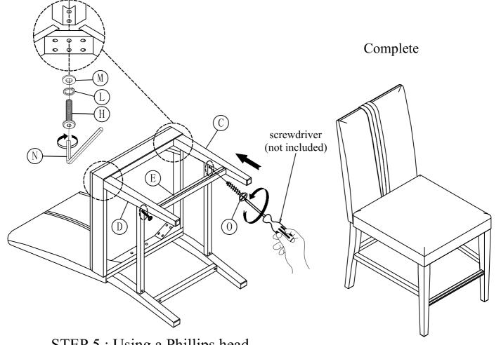
STEP 5: Using a Phillips head screwdriver tighten all screws.
