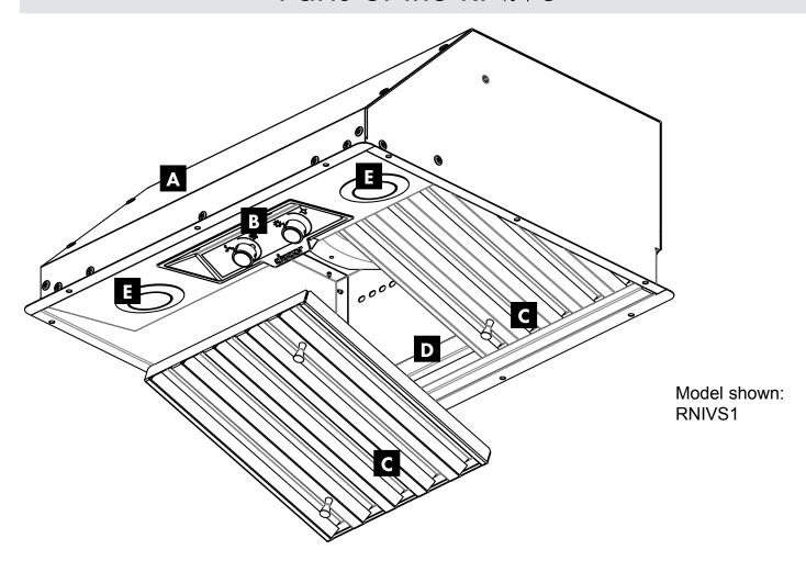
A RNIVS The Renassance® Integrated Ventilation System captures heat, smoke, and odors then moves them outside. This "range hood chassis" is without a canopy to fit inside custom designs.
