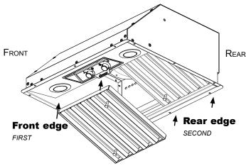
**Inserting the Filters**
