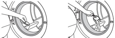
Single-dose laundry packets, Oxi-type boosters, color-safe bleach, or scented crystals can be added to the drum prior to adding laundry. When using single-dose laundry packets, make sure that the bulk dispenser is disabled or off (see Step 11).
