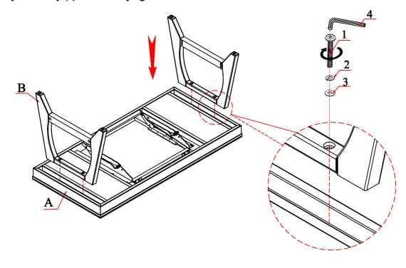
Step 2: Attach the Stretcher (C) to the Leg Frame (B) by using Flat Washer (3), Lock Washer (2) and Bolt (1). Secure well by Allen Key (4), fully tighten bolts at this time then attach the Wood plug (5).
