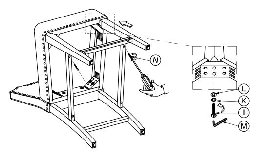
STEP 6: Using the Philips Head Screw driver to tighten all screws.
