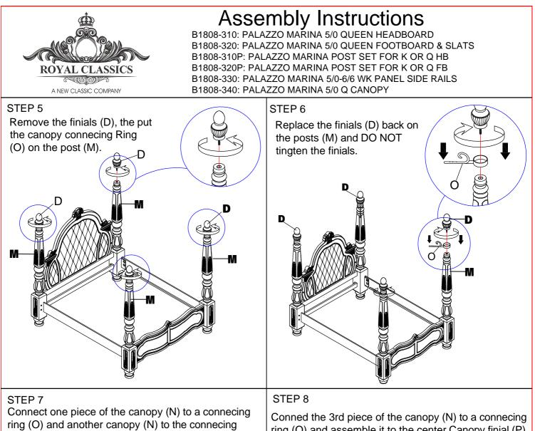
ring (O) and another canopy (N) to the connecting ring (O) directly diagianal to it. Then twist open the Canopy finial (P) in order to assemble the the two canopy (N) at the center by using Allen Key (19) with hardware 16, 17, 18.
