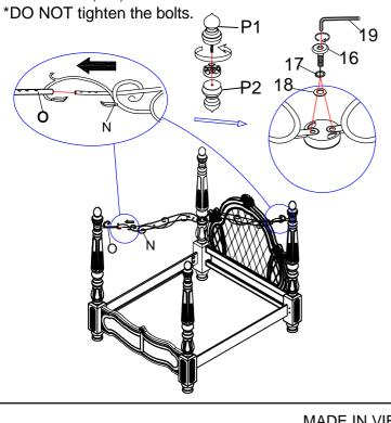
Conned the 3rd piece of the canopy (N) to a connecing ring (O) and assemble it to the center Canopy finial (P) using Allen Key (19) with hardware 16, 17, 18. \*DO NOT tighten the bolts.
