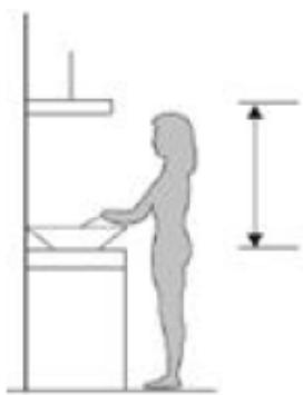
NOTE: The hood should be installed at a distance of 65cm (25.6") minimum to 76cm (30") maximum from the cooking surface.
