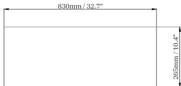
NOTE: Drill a hole in the cabinet measuring 830 x 265mm (32.7" x 10.4"). Make sure the distance between the edge of the hole and the front and rear edges of the cabinet is at least 35mm (1.4") to center the hood in the cabinet. The thickness of the cabinet should be limited to 15-25mm (0.6"-0.98") for best results.
