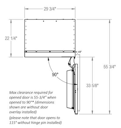
PLEASE NOTE: When installing column adjacent to wall, a 2" clearance is required if door opens towards the wall \*90° achieved when included hinge stop pin is installed. Pin must be installed prior to full integration
