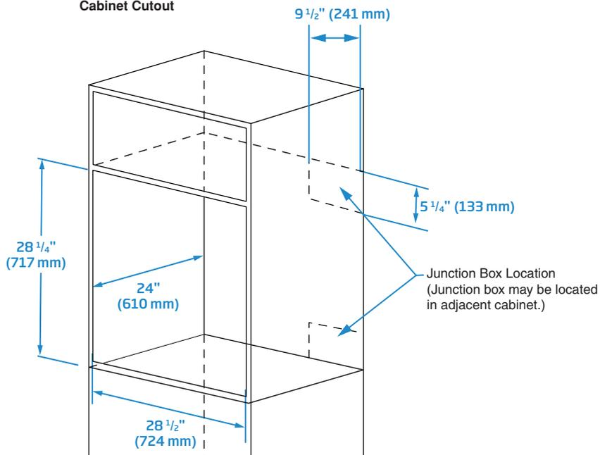
If installing in lower cabinet, leave 4" (102 mm) minimum clearance below.
