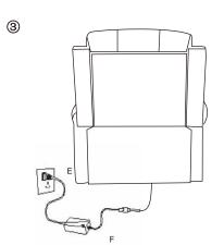
3. Connect the connector from motor to the power cord and transformer
